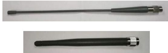
Figure 4-3-1 UHF Radio Antenna (Above) and 3G/GPRS Antenna (Below)
